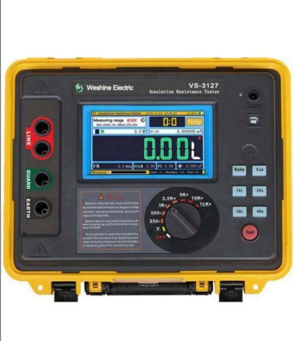
measurements up to 15 kV test voltage with a maximum resistance of 30 TΩ. Resistance measurement accuracy is ± 5 % from 1 MΩ to 3 TΩ! For utilities and service companies the VS-3127 is an all-around tester with its flexibility and future proofing capability. The
